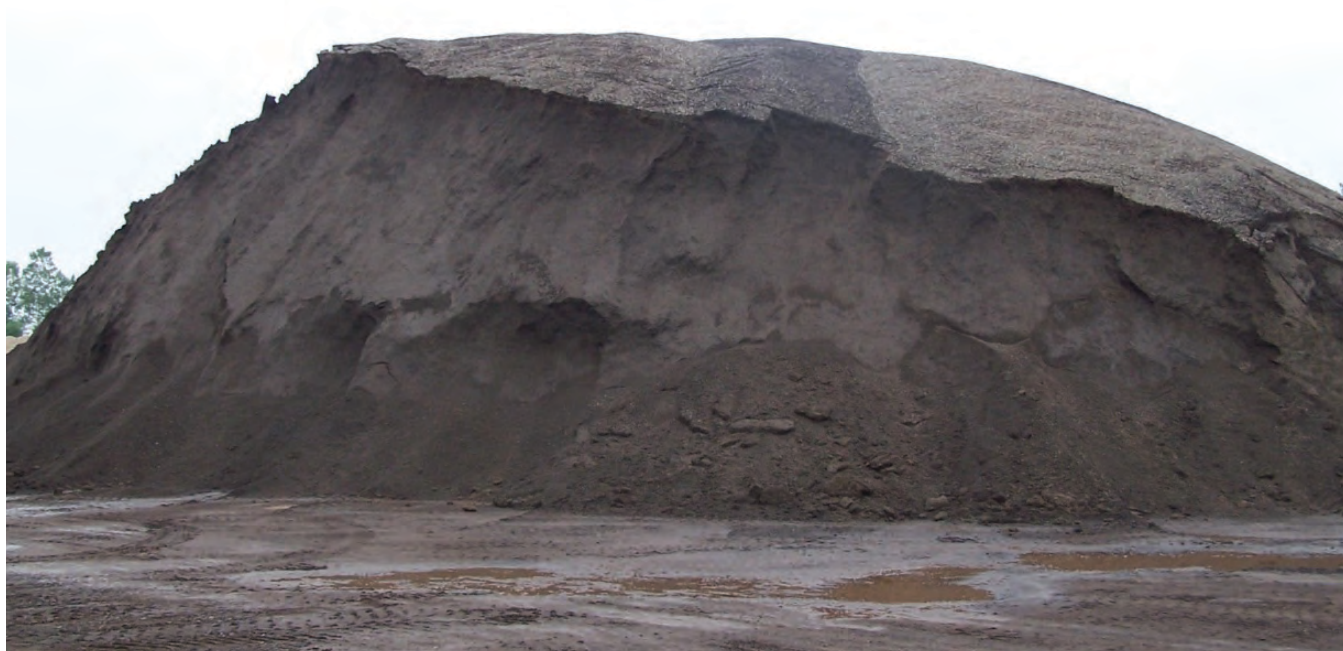
Figure 3-1. Processed RAP with a uniform appearance.
