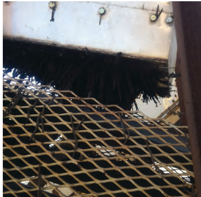
Figure 5-3. Magnet used to remove nails from RAS feed to the asphalt plant.
