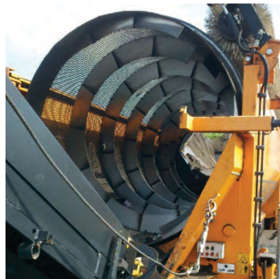
Figure 5-1. Shingle grinder (left) and rotating Trommel screen (right) used for RAS processing.
