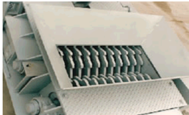
Figure 2-10. Roller crushers designed to break up agglomerations of RAP.
