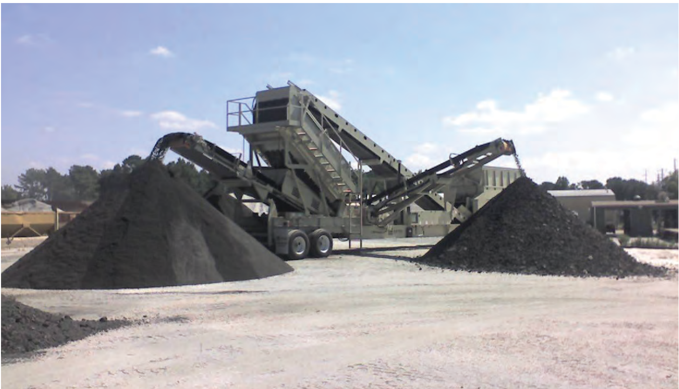
Figure 2-7. Portable RAP fractionation unit. This unit screens RAP into three sizes: +3/4 " on right, -3/16 " on left, and 3/4 " \times 3/16 " in back.
